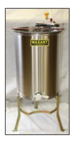
Your extractor is ready to use straight out of the box. We recommend running warm soapy water through it before its first use. If you ordered a leg kit, assemble and bolt it to the extractor. Your extractor is belt driven, and you should expect 15+ years of enjoyment before replacing the belt.
