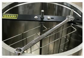
REMOVE HAND PULLEY SHAFT/BOLT USING A 3/4" WRENCH THERE IS A BOLT UNDER THE COLLAR AND UNDER THE TOP BAR
