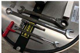
TOOLS NEEDED: 7/16" SOCKET AND/OR WRENCH 1/8" ALLEN WRENCH 3/4" WRENCH AND/OR ADJUSTABLE WRENCH
